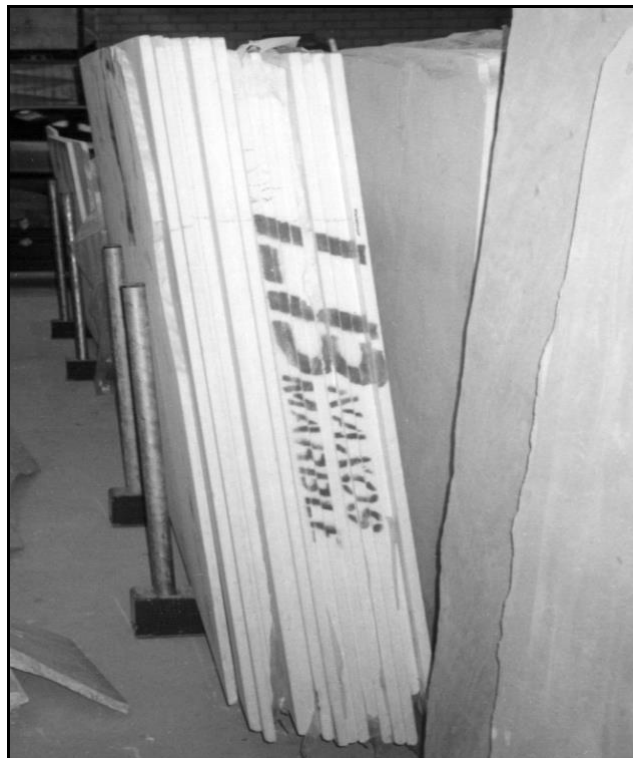
Picture 6.5 – Example of a too little clearance angle with a too large overall thickness of the slab.
