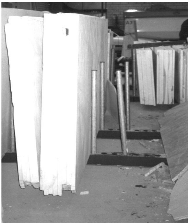
Picture 6.4 – Example of too little clearance angle with too large overall thickness of the slab.
