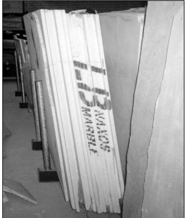
Picture 6.5 – Example of a too little clearance angle with a too large overall thickness of the slab.
