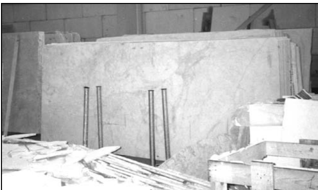
Picture 6.6 – Overloaded iron support tubes showing risk of breakage respectively crushing.
